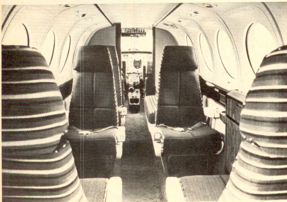
Super King Air cabin is extremely quiet, seats 9-12 depending upon interior configuration. The 6-psi pressurization system limits cabin altitude to 6,700 feet at FL 250.
